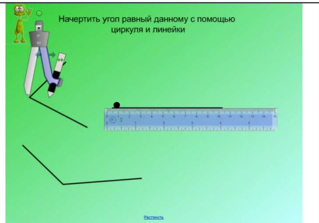
*Pressing a smaller leg of compasses, we can establish distance, convenient for us, between compasses legs*
